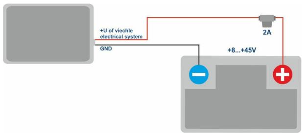
Figure 3 - Standard connection layout of the tracker
