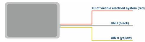
Figure 2 - Color marking of the tracker wires
